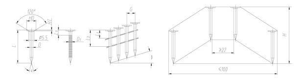
HD – Head Diameter, d – shank Diameter, HT – Head Thickness, L – Length, D1 – Ring Diameter, L1, L2 – Welding Position L3 – Head to Ring Space, a – Point Angle, ß – Shear Angle, H – Coil Height, G – Nail Gap
